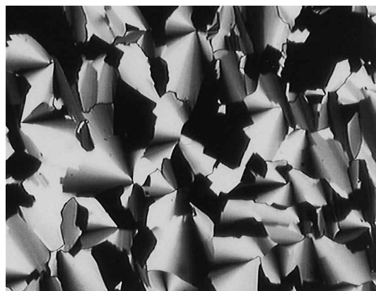
Figure 3. Polarized optical microscopic texture observed at the transition from the induced columnar to the cubic phase of the binary mixture of compounds 2 and 1.14 ( x_{1.14} = 0.9 ) at 136°C.
